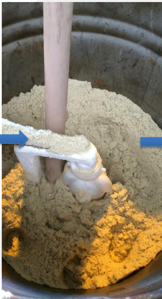
manual sand filling of a molding box
