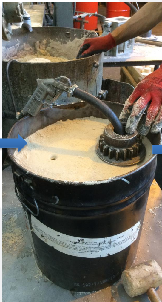
blowing through the sand with CO2
