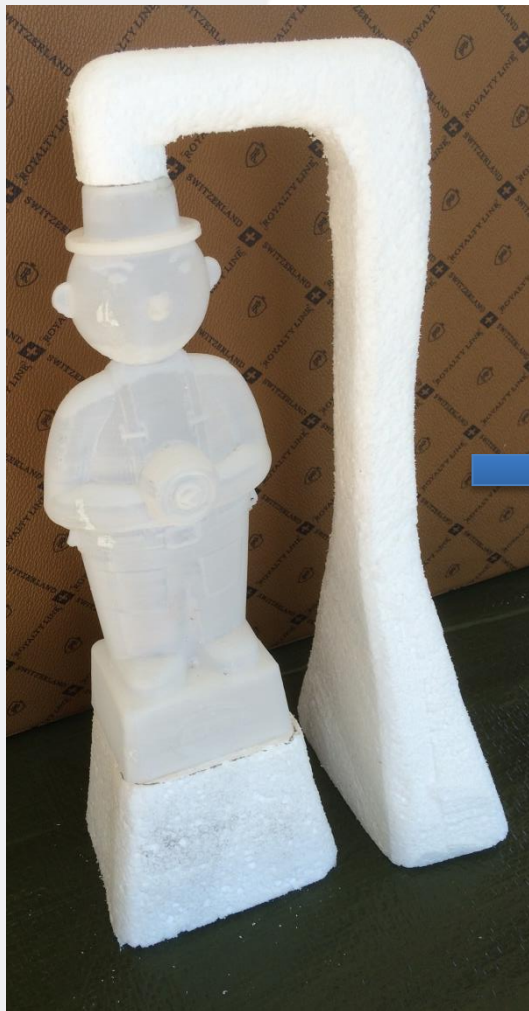
gating system cut out of foamed polystyrene
