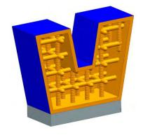
Creating hollow parts with internal support structure + machining
